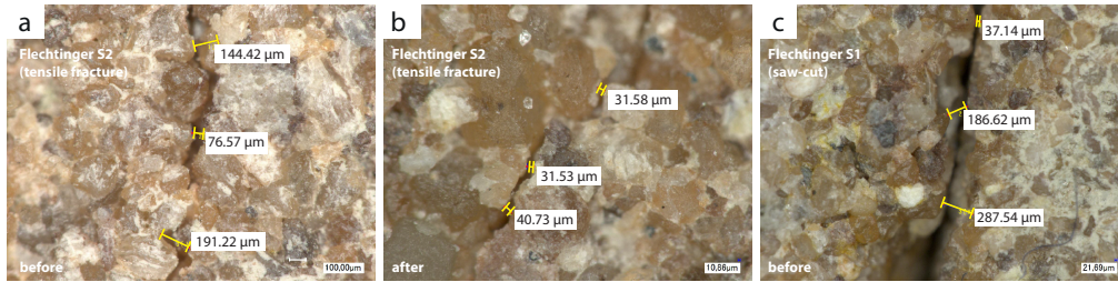
Figure 3: Optical aperture of tensile fracture before and after testing (a,b); and the saw-cut (c).
